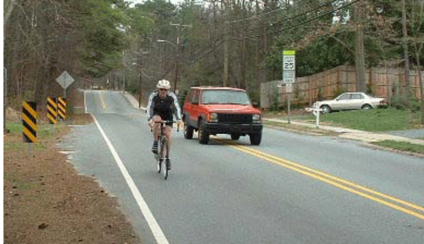
Figure 4. In a 10-foot lane, bicyclists are considered to have the same capacity impact as 1.0 cars.
