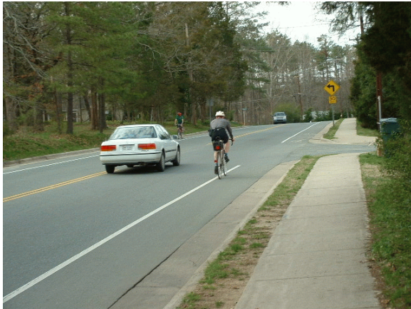
Figure 1. A 4 ft BL with 12 ft standard lane.
