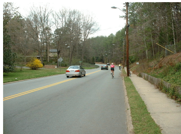
Figure 2. Encroachment without conflict in a 15 ft WCL. This was not a necessity but a simple courtesy of the motorist.
